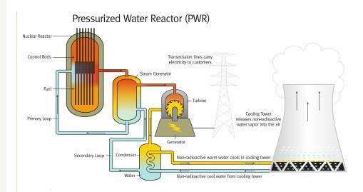
Davis-Besse Nuclear Power Station produces electricity much like a coal power plant. The main difference is the type of fuel used. The fuel used in a nuclear plant is uranium.
